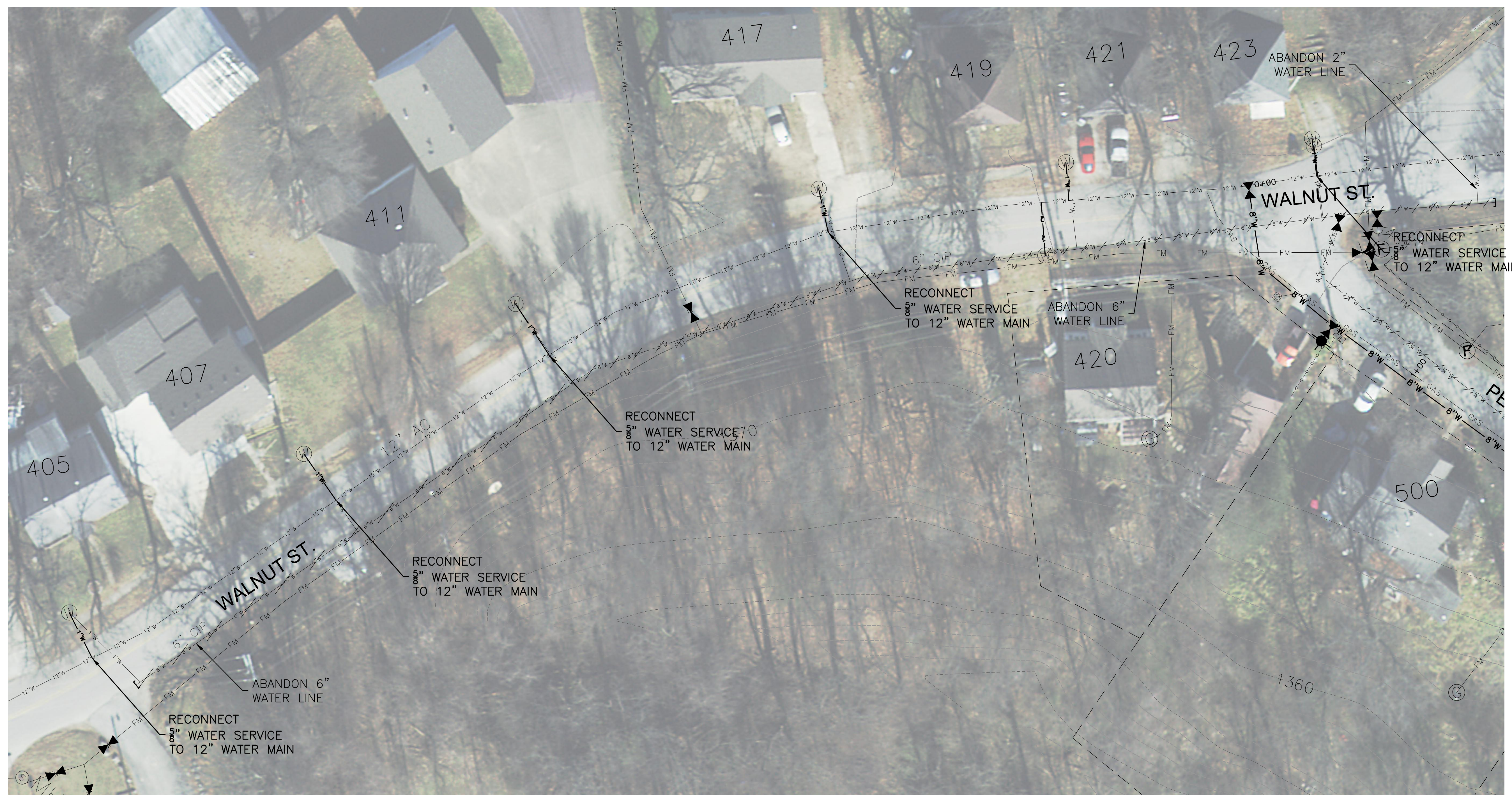
PLAN – MOVE WATER SERVICES FROM 6" MAIN TO 12" MAIN ON WALNUT STREET SCALE: 1"=20'
