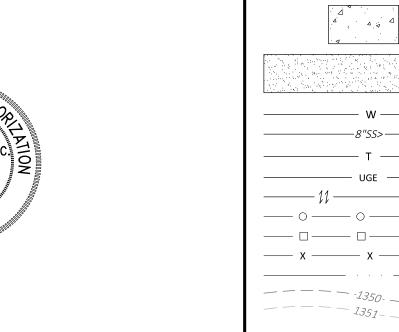
Ex. Road Centerline — Ex. Easement Line Ex. Concrete Ex. Gravel Ex. Water Line Ex. Sanitary Sewer Line Ex. Telephone Line UGE — Ex. Underground Electric Line — [] ——— Ex. Overhead Electric Line —— O —— O —— Ex. Chain Link Fence Line — X — X — X — Ex. Wire Fence Line Ex. Contours Ex. Fire Hydrant Ex. Water Valve Ex. Sewer Manhole Ex. Gas Meter Ex. Electric Meter Ex. Electric Transformer
